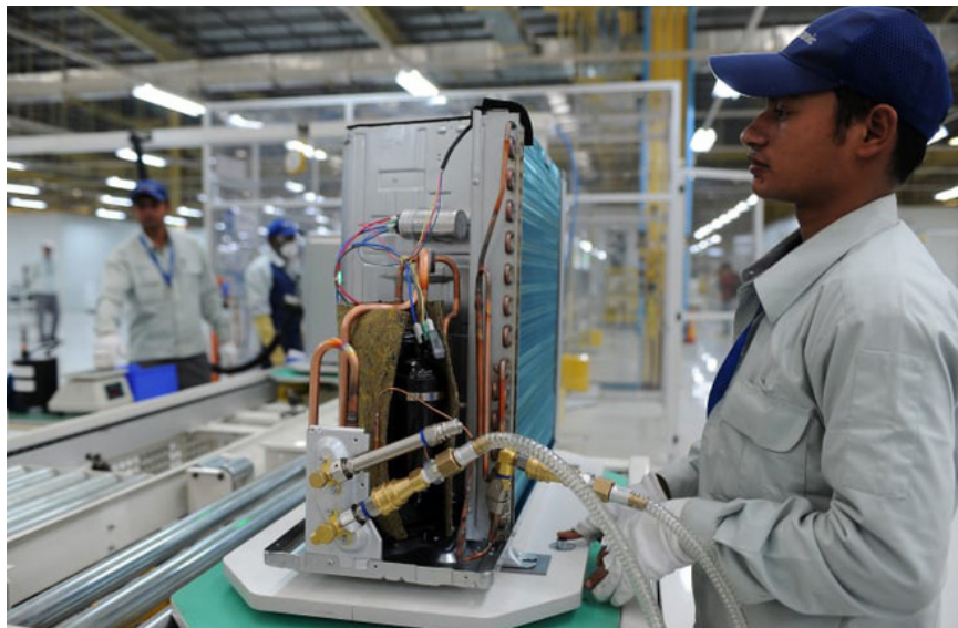
An air conditioner is assembled at a factory in Jhajjar, India.
