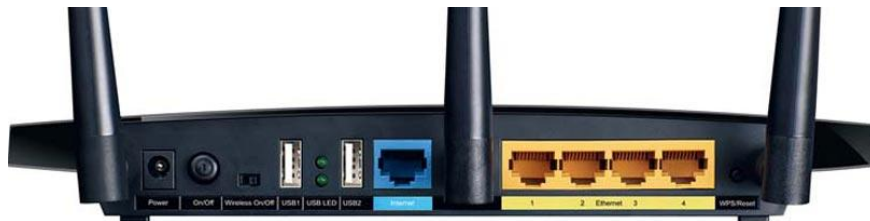
Figure B : The back of TP-Link's Archer C7 AC1750 router includes a set of RJ-45 ports like a hub or switch
