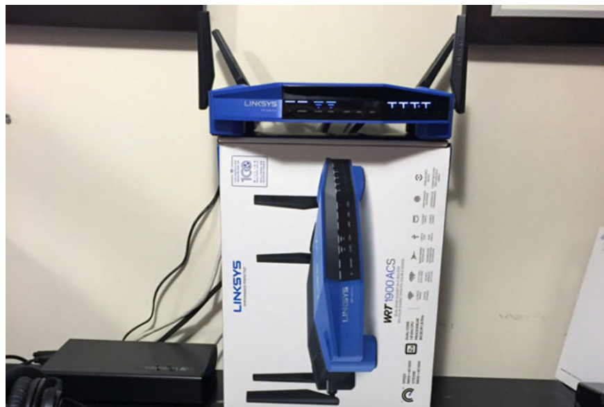
4. Configuration 4: Same as (3), but the front antenna is set at an outer angle of 45 degrees compared to the rear antenna.
