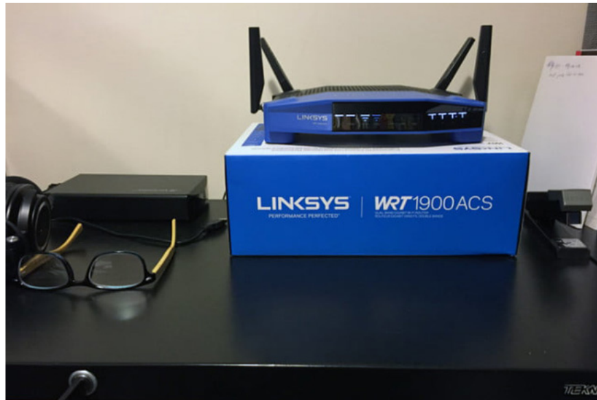
3. Configuration 3: Same as (1) but the router is placed on the cardboard box vertically placed about 12.5 inches from the cabinet.
