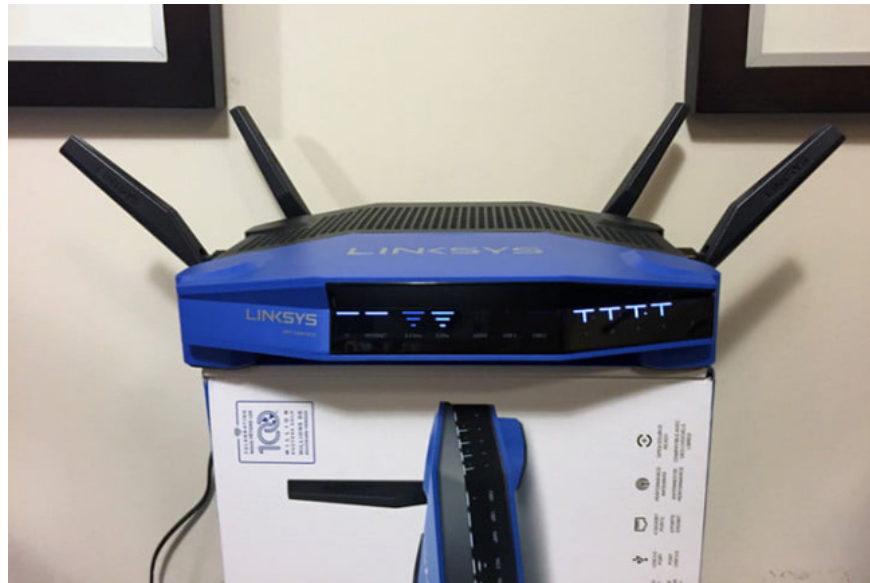
5. Configuration 5: Same as (3) but the front antenna is set at 90 degrees outside (parallel to the floor).
