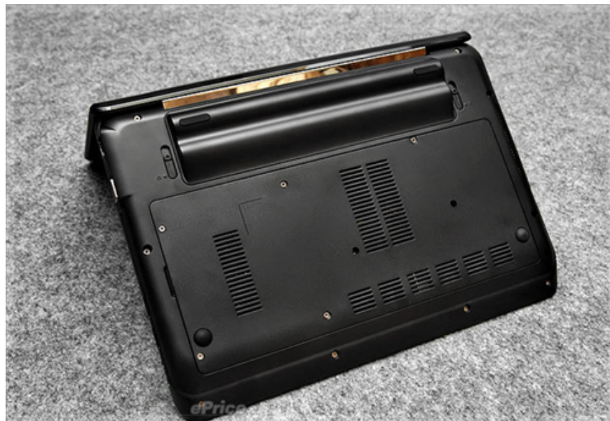
ViewBook ??130 (770 USD) - 13.3 inch, resolution of 1366 x 768 pixels, Intel ULV 743 1.3 GHz, RAM 2 GB, HDD 320 GB, Intel GMA 4500MHD, 1.45 kg.
