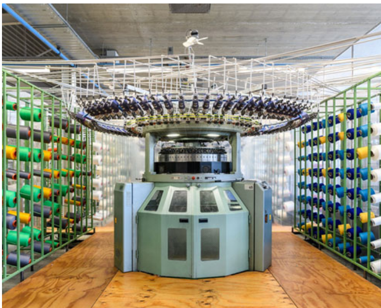
A knitting machine has about 4,000 needles at the Kvadrat Febrik textile factory in Tilberg, Netherlands.
