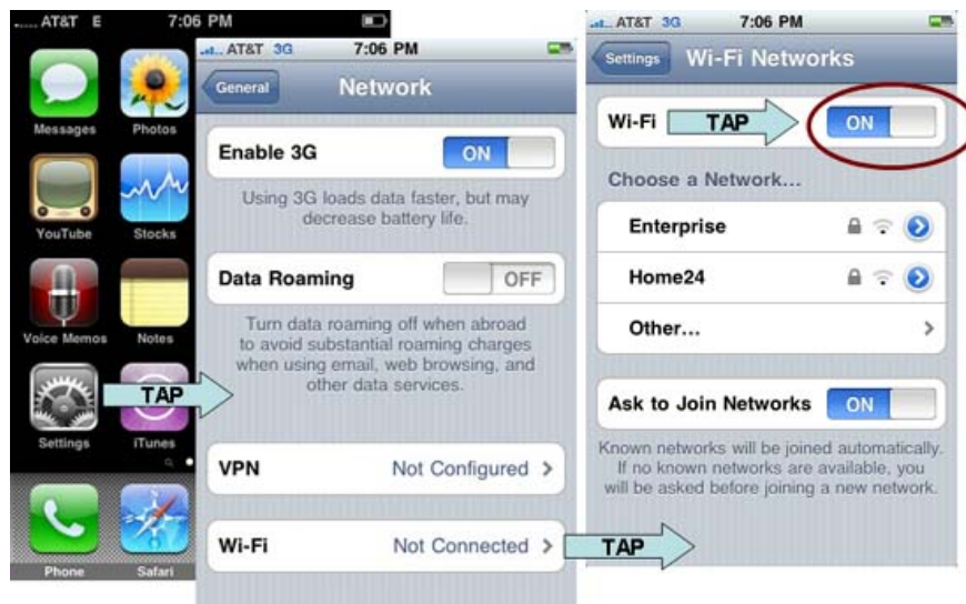
Figure 1: Verify that the client's Wi-Fi is turned on
