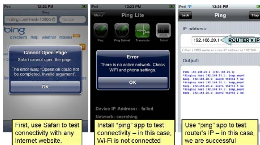
Figure 3: Sending test traffic using Safari or Bing
