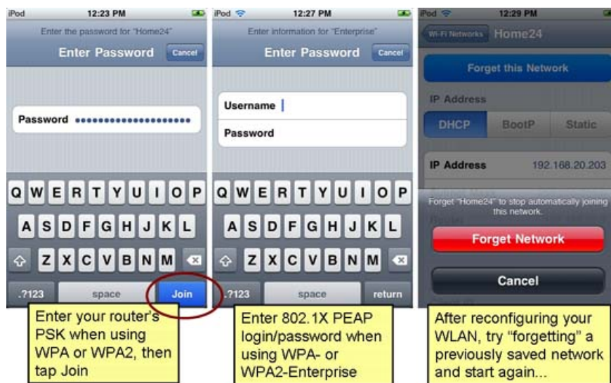
Figure 4: Matching security settings between the client and the router
