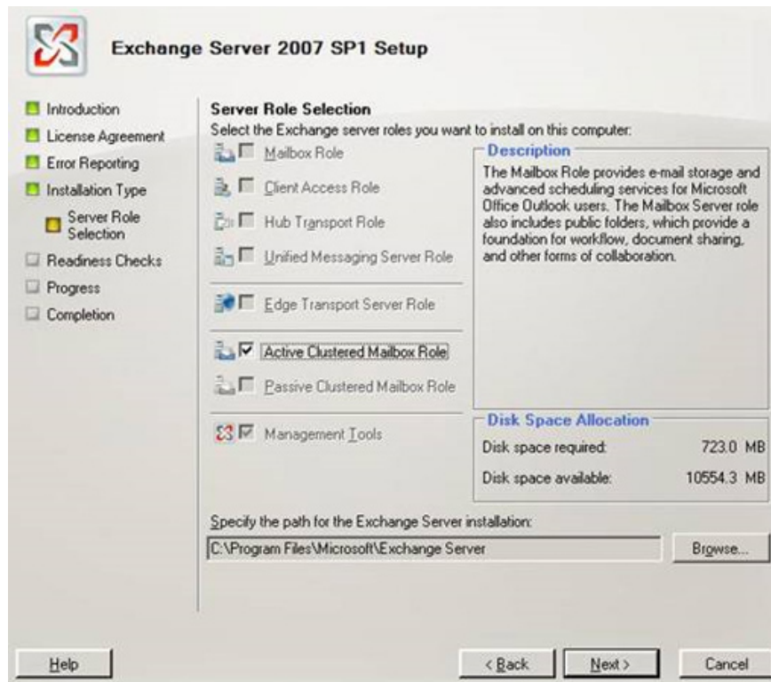
Figure 3: Installing Active Clustered Mailbox Role.
