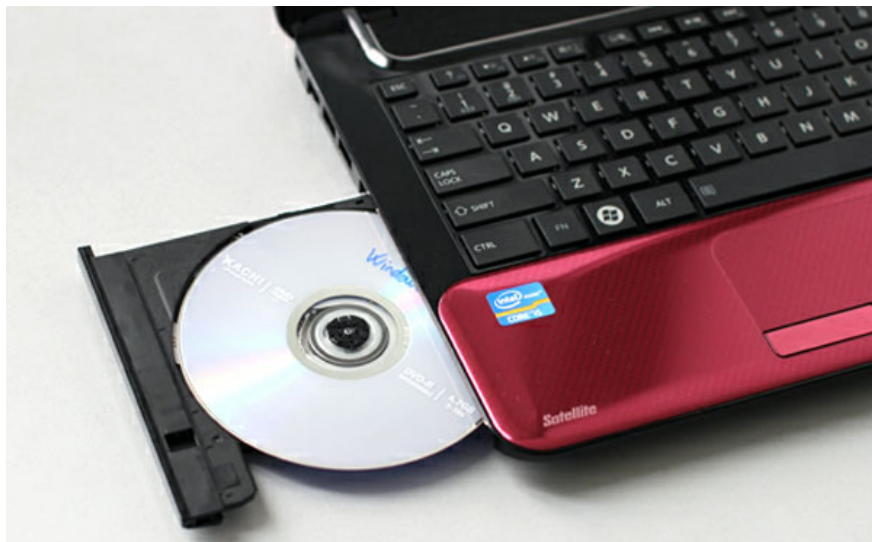
The M840 is one of the few laptops that has the left optical drive design.
