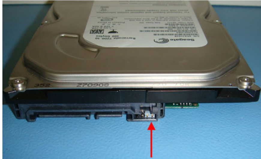
Figure 9: Hard disk drive with SATA-150 / SATA-300 jumpers being placed in 'SATA-150' position
