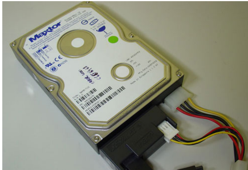
Figure 7: Standard IDE drive 'converted' to Serial ATA via one adapter Jumper SATA-150 / SATA-300
