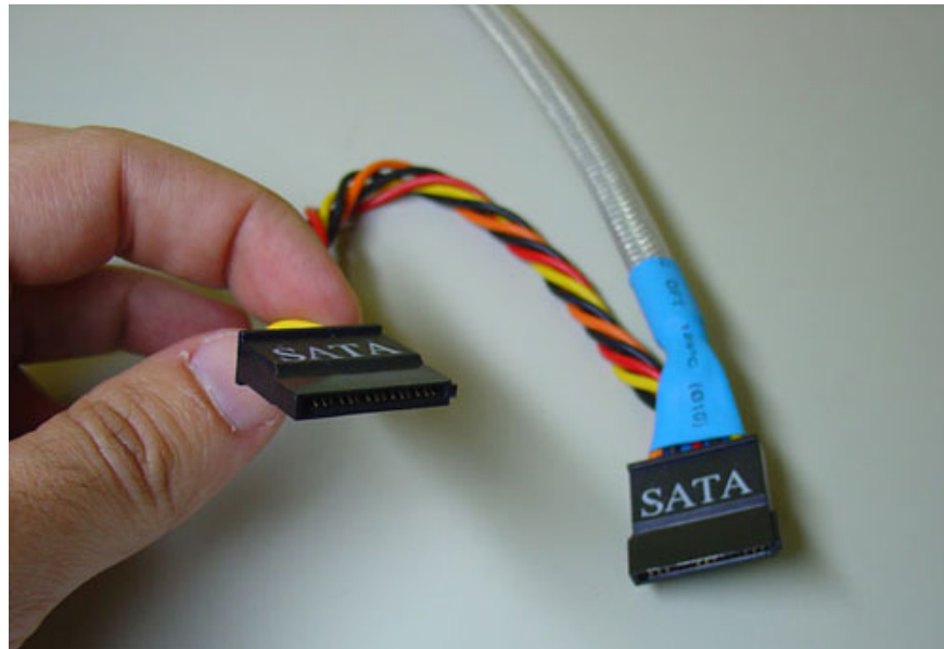
Figure 5: Serial ATA power connectors on ATX12V power supplies
