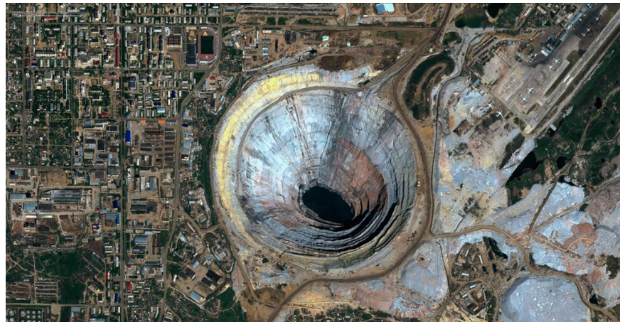
Opened diamond mining mine Mir, Siberia, Russia. The mine was deactivated after 44 years of diamond exploitation and became the second largest artificial pit in the world with a depth of 525m and a diameter of 1,200m.
