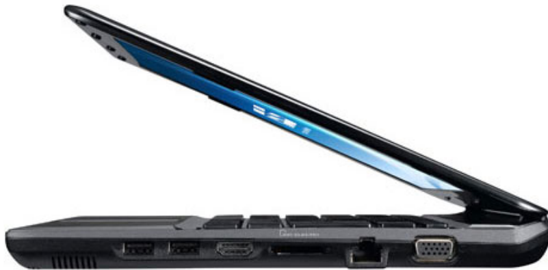
The machine is fully equipped with connectivity ports such as HDMI, LAN, USB .
