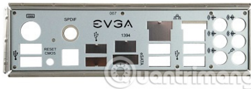
Plate I / O shield for EVGA motherboard
