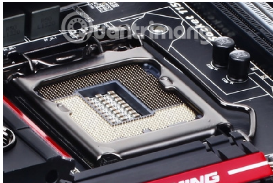
Intel LGA 1150 socket on Gigabyte motherboard
