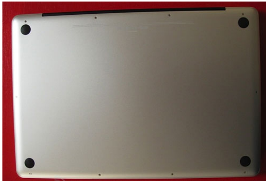
On the bottom, the battery is in the machine, so there is no place to remove the battery cover as usual.
