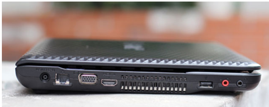
Left side with LAN port, VGA, HDMI, heat sink slot. The device has no USB 3.0 port
