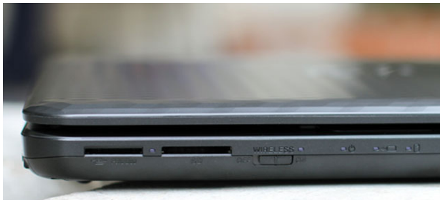
Front edge with MS and SD memory card reader, Wi-Fi on / off switch.
