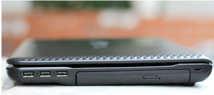
Right side with optical drive and 3 USB ports.
