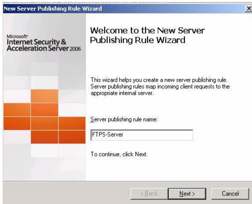
Figure 1: Name the new Publishing Rule on the Welcome page of New Server Publishing Rule Wizard.
