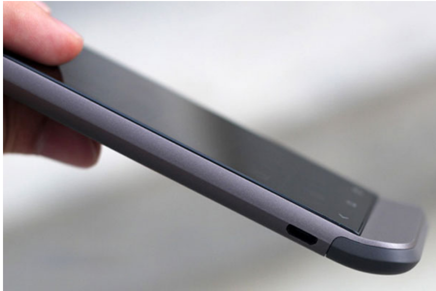
The case is made of monolithic aluminum with the tail section under the bend screen. (Photo: Tuan Anh).
