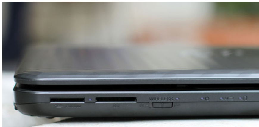
SD card reader at the front edge. (Photo: Tuan Hung).
