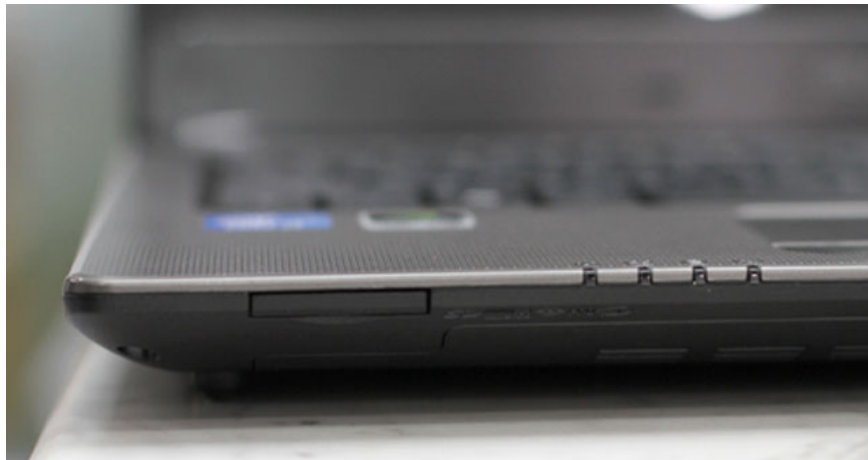
Front edge with SD memory card reader.
