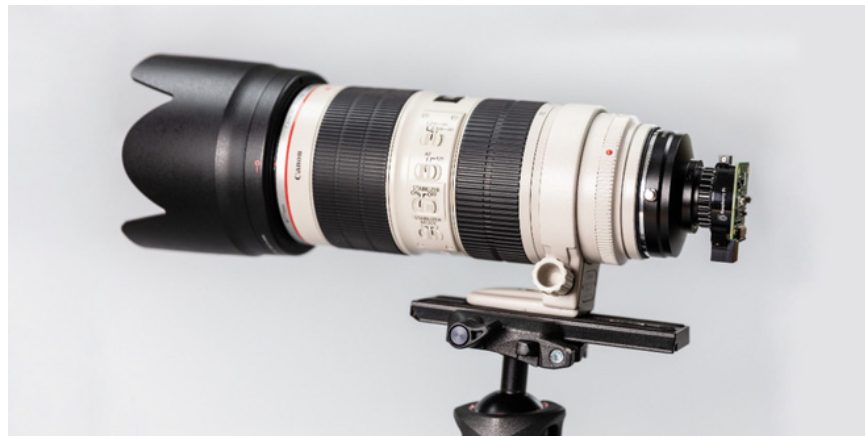
High Quality Camera Module with Canon 70-200mm f / 2.8 lens.
