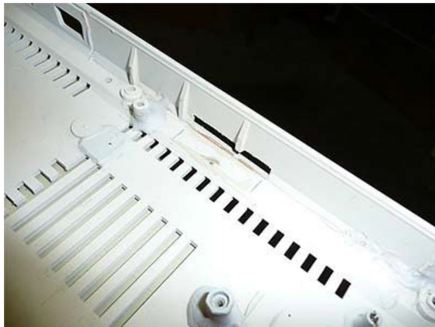
A large enough slot is inserted to hold the CF card.
