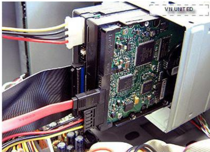
IDE (left) and SATA hard drives (right) on the same tray.
