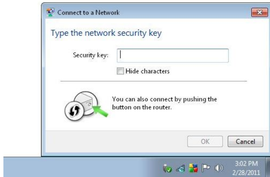
Figure 1: Prompt to enter the PSK key or press WPS on the router.
