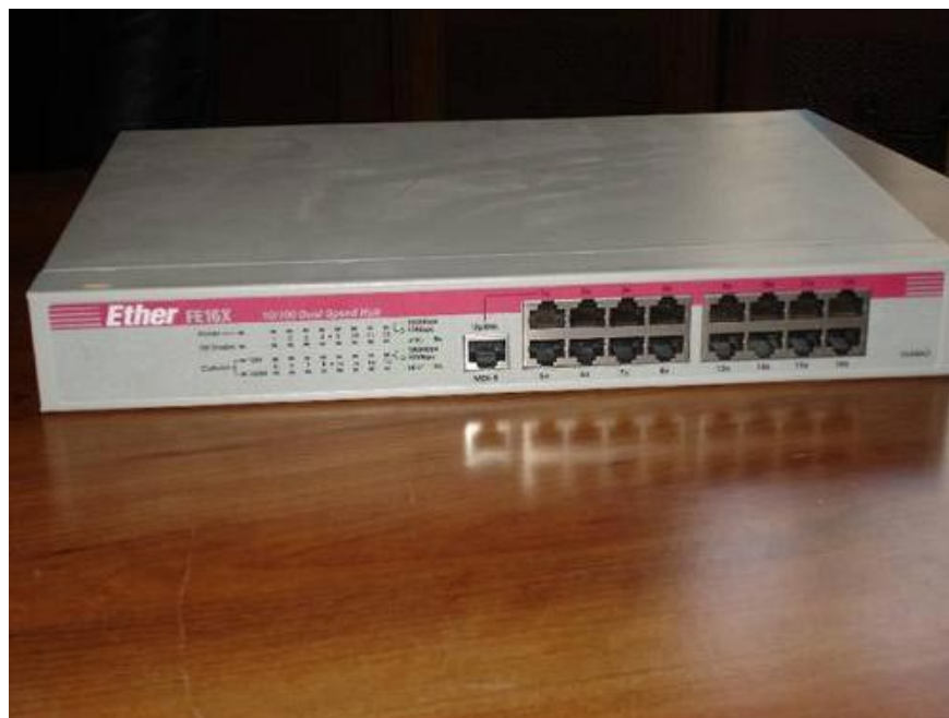
Figure 3 : Hub is a device that acts as a central connection point for computers on a network.
