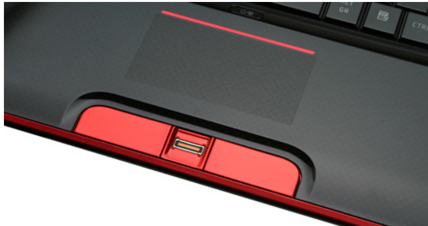
Multi-touch touchpad and fingerprint identification slot.
