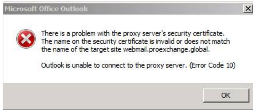
Figure 13: Outlook Anywhere fails when connecting because the name of the security certificate does not correspond to the name of the target site.
