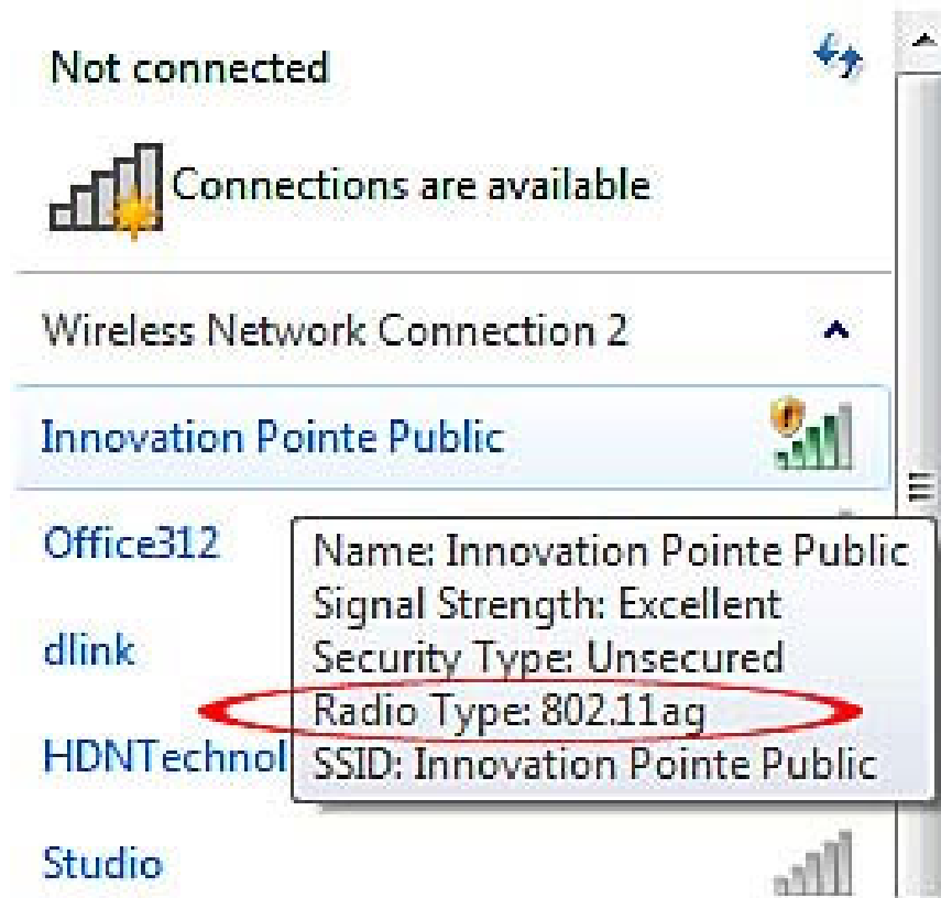
Figure 2: This connection works with both 2.4GHz Wifi Adapter (802.11g) and 5GHZ (802.11a)
