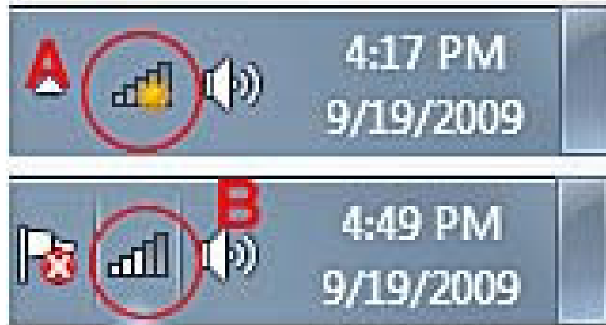
Figure 6: Detecting some Wi-Fi networks but no connection has been established (A). A Wifi connection is being used (B).
