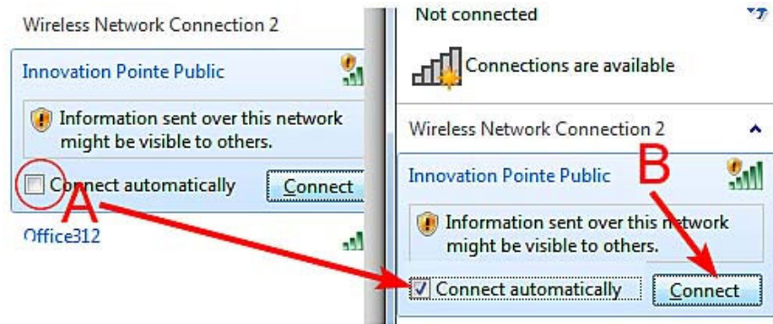
Figure 3: Save an open Wifi connection for the next use (A) and connect to the open Wifi network (B).
