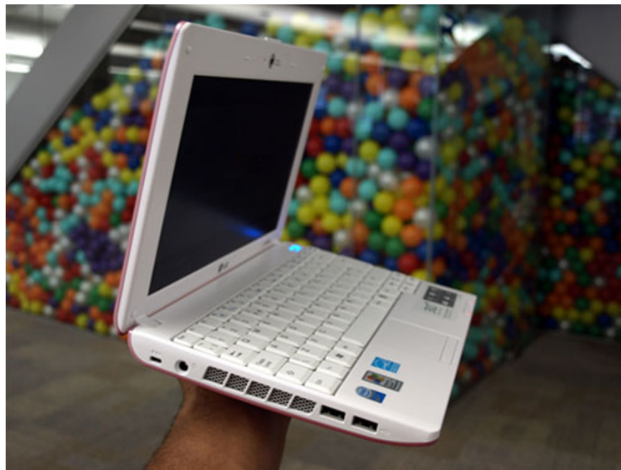
On the left side, there are clearly two USB ports, air vents to reduce heat for the Atom N270 processor.
