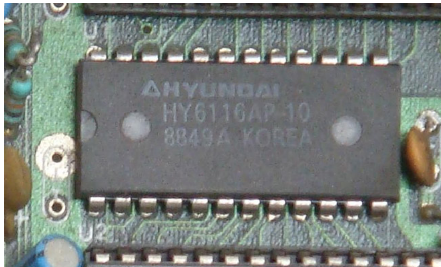
A static RAM chip from a copy of Nintendo Entertainment System (2K x 8 bits). Photo source: Wikipedia
