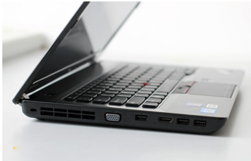
Left edge with USB 3.0 port, USB 2.0, HDMI, VGA.
