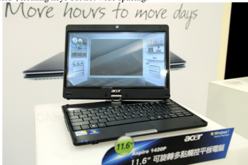
Chiclet keyboard "hybrid", floating keys but not wide spacing.
