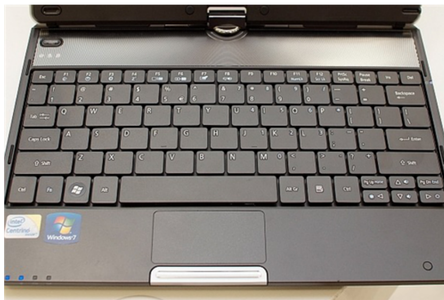
Chiclet keyboard "hybrid", floating keys but not wide spacing.
