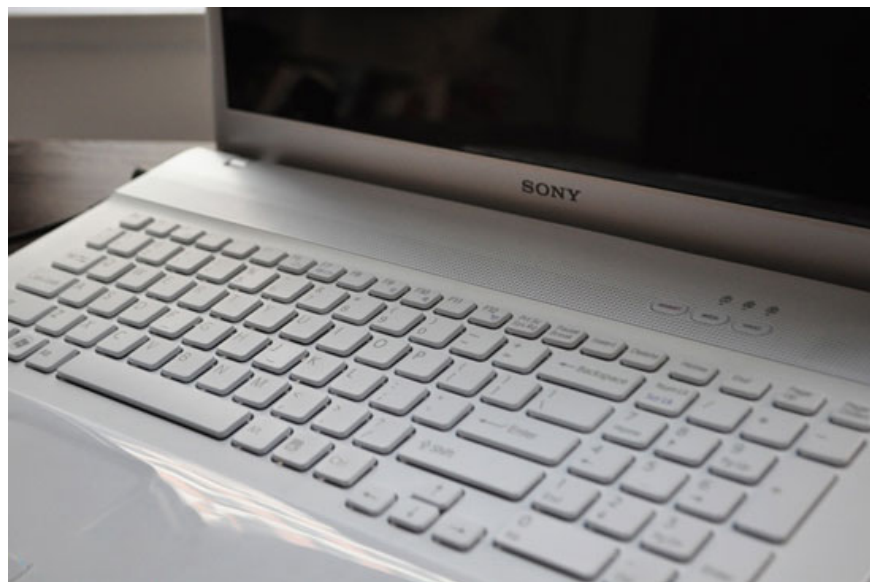
Chiclet keyboard with full size and extra numeric keypad on the right.
