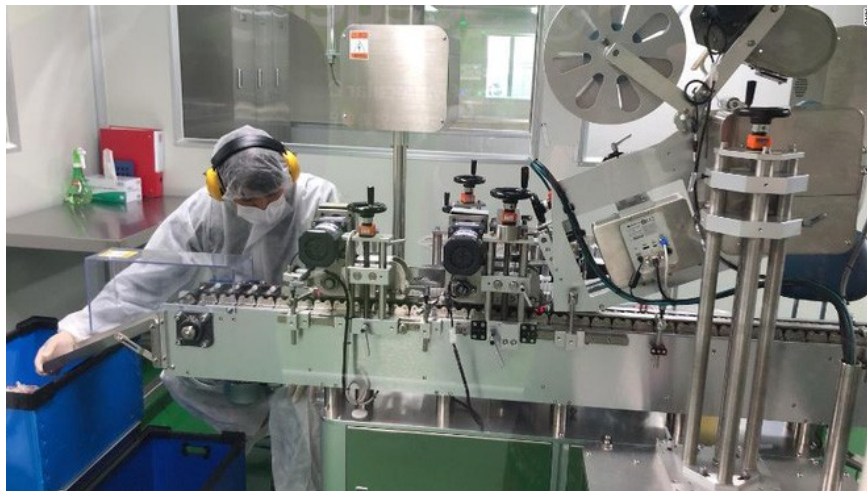
A worker at Seegene oversees a labeling line for the test kit vial.
