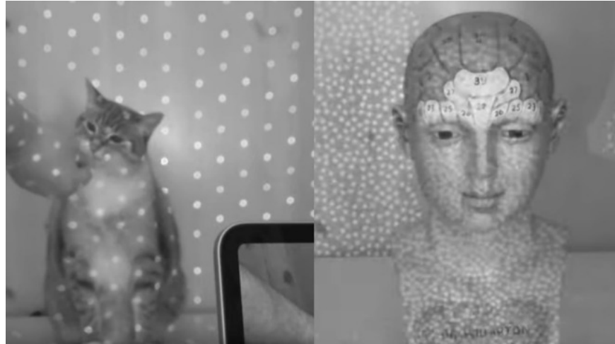
Infrared dots from LiDAR (left) and Face ID (right)
