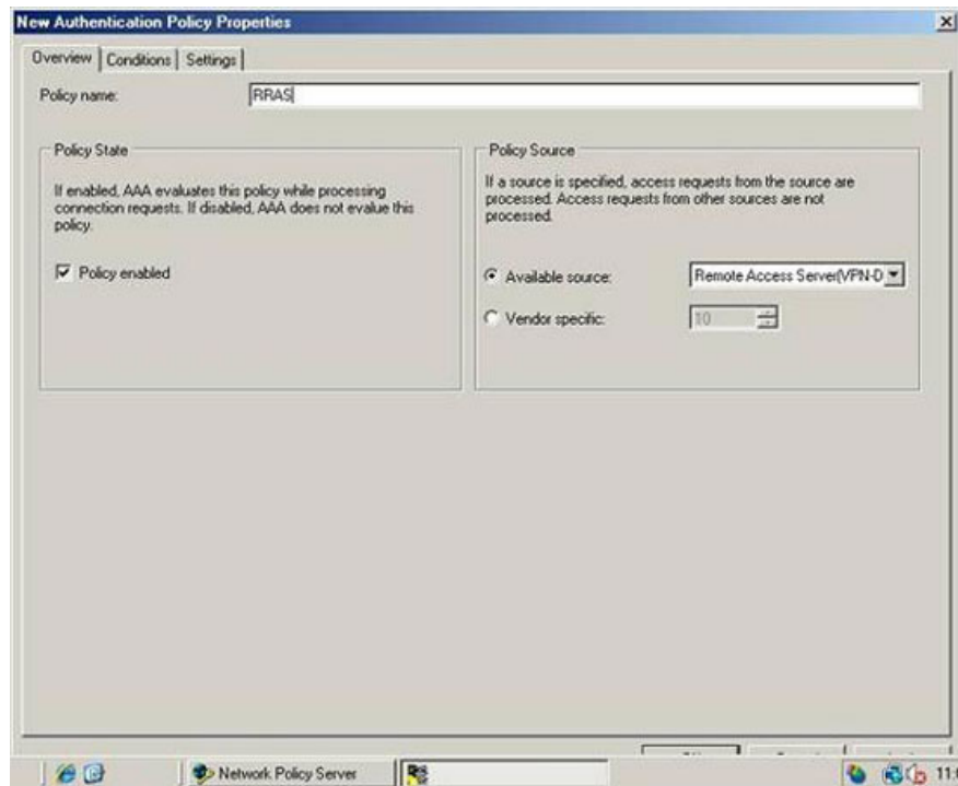
Figure A : Enter RRAS as a policy name and then verify that policy is enabled
