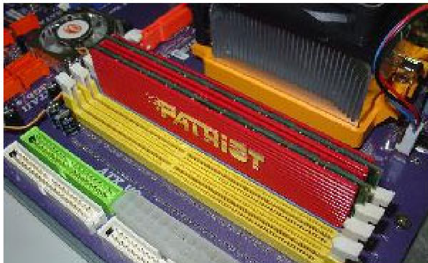
Figure 8: Memory modules are correctly installed in dual channel mode.
