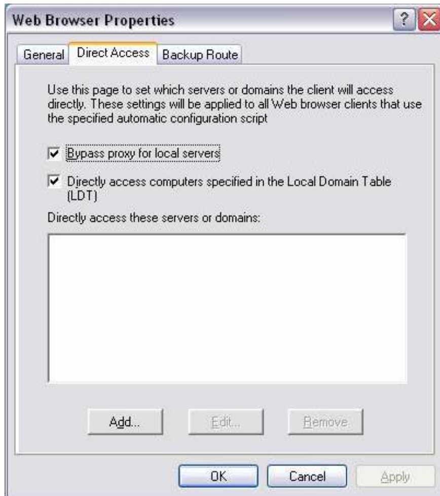
Figure 4: Configure the parameters provided for the Web proxy client on ISA Server
