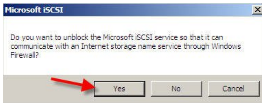
Figure 13: Windows Server 2008 - Allow iSCSI via Firewall
