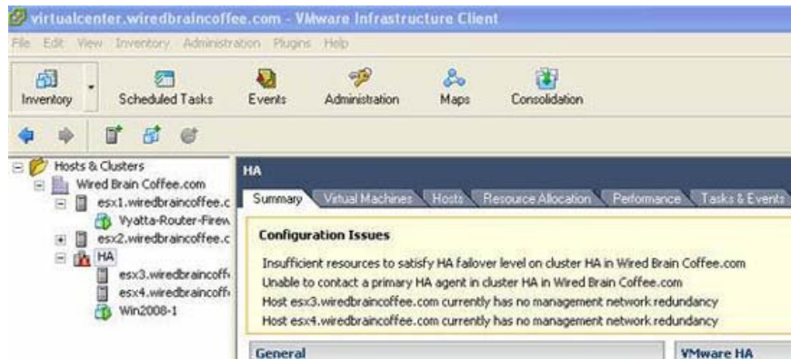
Figure 3: Configuration problems because there is no network management VMware redundancy
