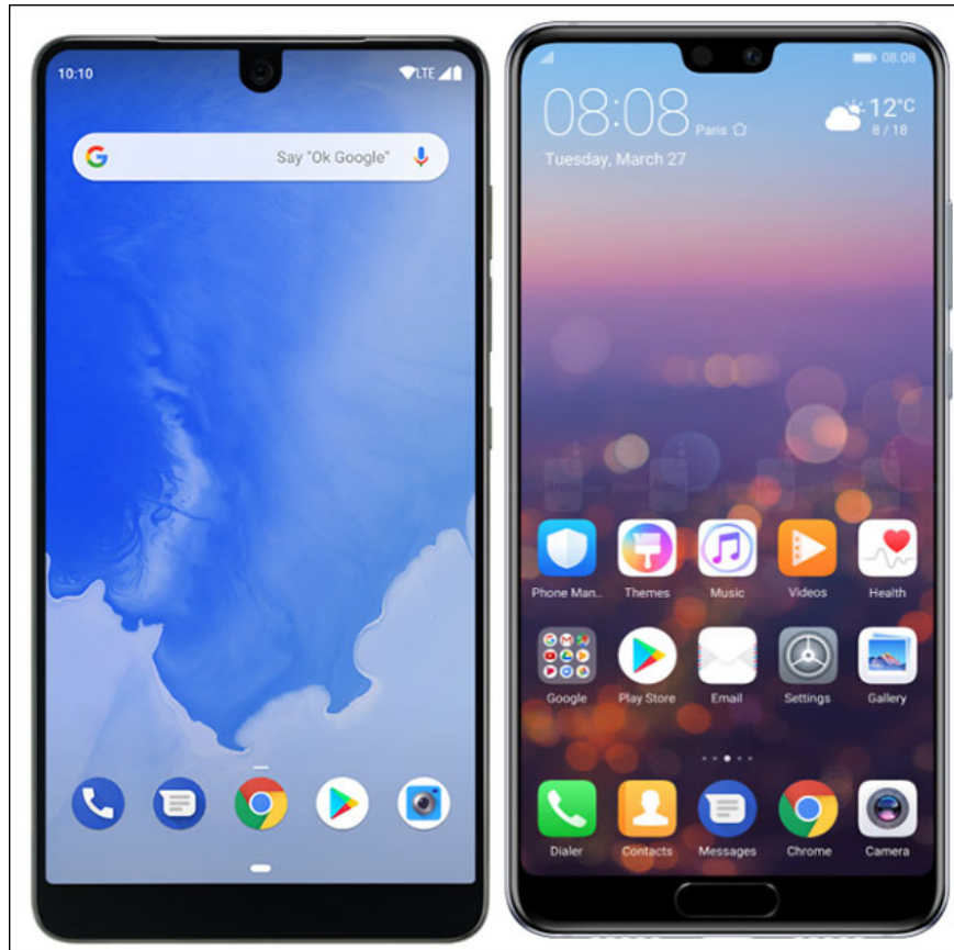
Examples of grooves on Android: Essential PH-1 (left) and Huawei P20 (right)
