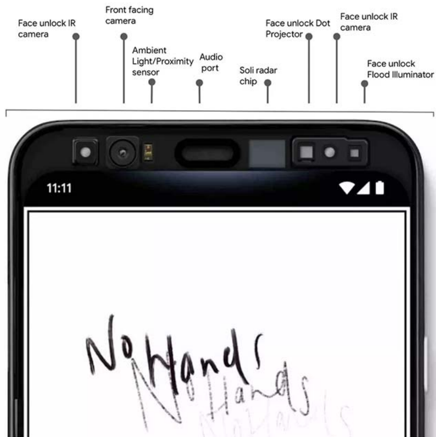
List of sensors, processor chips are equipped on Pixel 4
