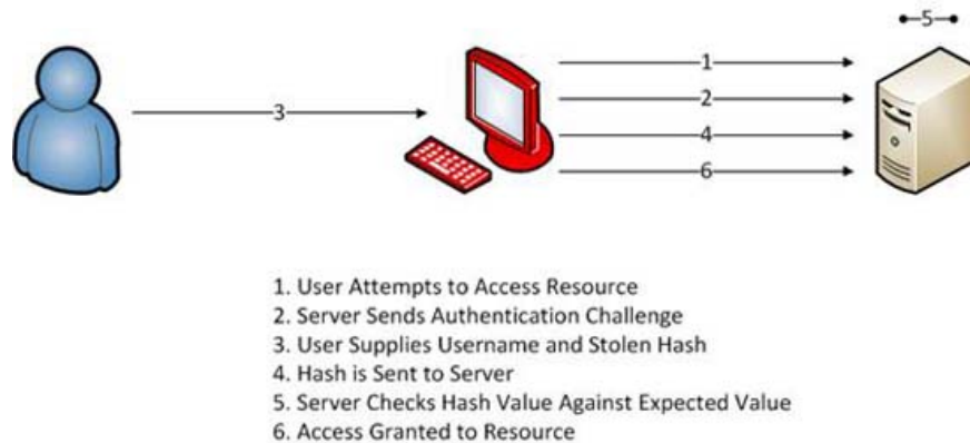
Figure 2: Pass the hash directly to the destination host
