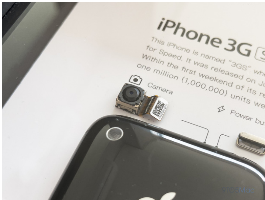
3MP camera cluster with autofocus and 480p video recording.
