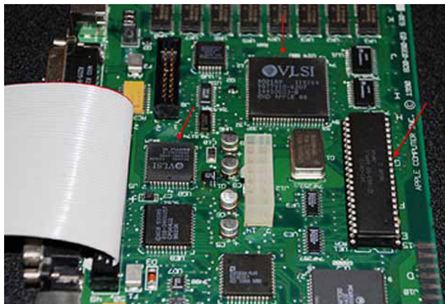
The upper part of the motherboard, one can see VLSI chips.
