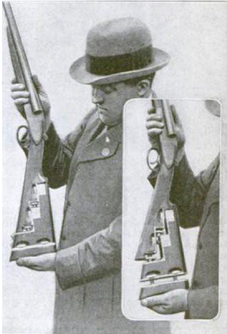
A custom stock and shock absorber designed for female athletes. The gun stock can be extended or shortened according to the needs of the user thanks to the set screw design.
