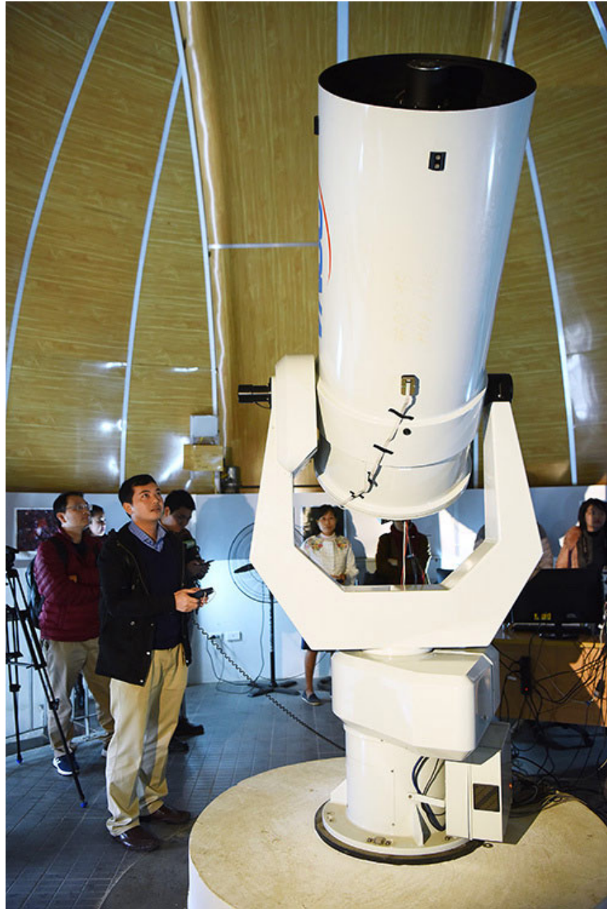
This is a viewfinder that can be viewed at a wide angle, used to shape and move the subject to capture / aim at the field of view of the telescope tube.
