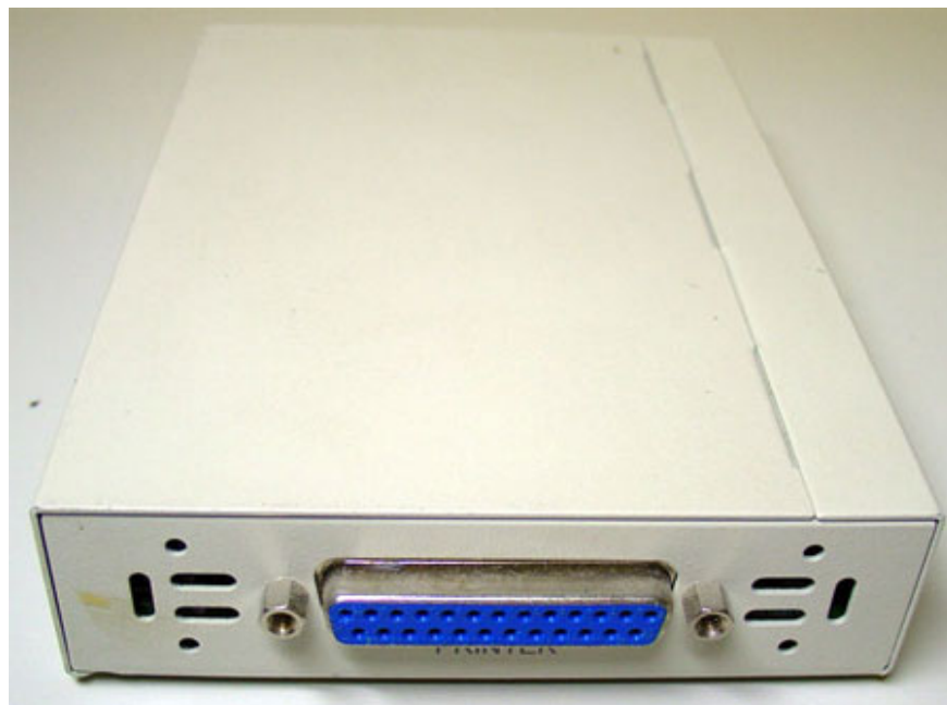
Figure 2: Parallel port on a router with the print server feature
