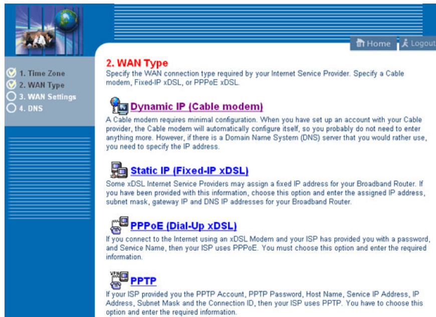
Figure 14: Basic installation, second screen (connection type)
