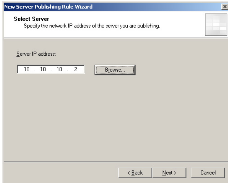
Figure 18: Enter the IP address for the server on the Select Server page.
