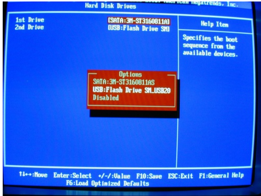
Figure D: When UFD is plugged into a USB port, you can configure UFD as a boot device
