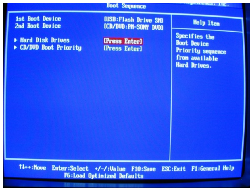
Figure E: Boot Sequence screen The UFD indicator is set to be the first boot device
