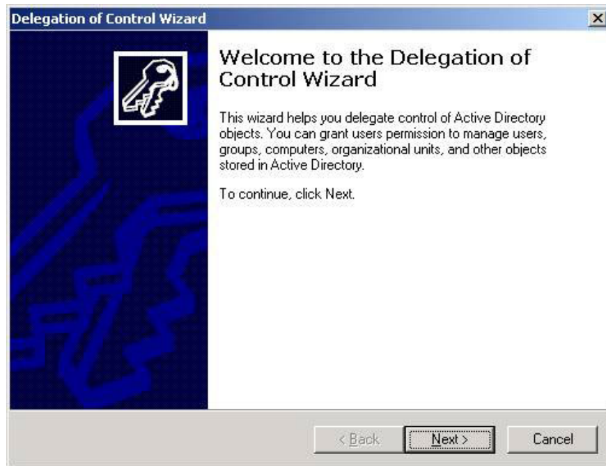
Figure 6: The Delegation of Control Wizard allows you to easily configure the permissions on Active Directory Objects
